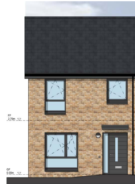
FRONT ELEVATION FACING BRICK
