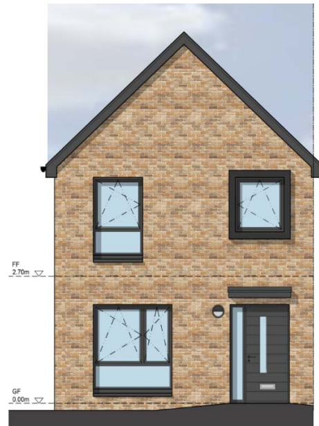
FRONT ELEVATION FACING BRICK
